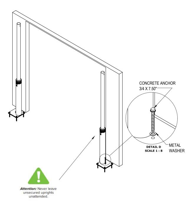
(8) USING A SCISSOR LIFT, SLIDE COUPLERS ON THE CROSSBAR ENDS, AND SLIDE ONTO POSTS.
