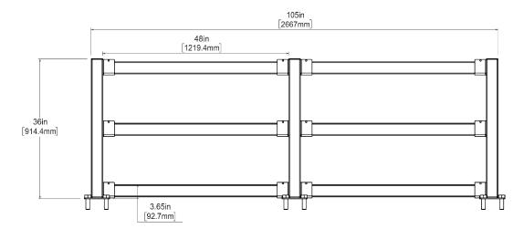
Steel cross members safely protect critical systems, yet easily removed to allow access for maintenance
