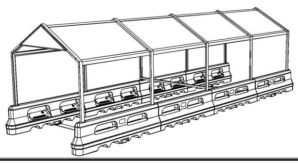
**IMPORTANT:** Assemble on a flat, level surface. All cart corrals should be inspected on a regular basis for damage. McCue recommends a minimum of two inspections per year in the spring and fall. Any damaged pieces, including ground frames and lane dividers which are not flat and flush with the ground, should be replaced with McCue replacement parts.
