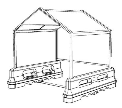
**IMPORTANT:** Assemble on a flat, level surface. All cart corrals should be inspected on a regular basis for damage. McCue recommends a minimum of two inspections per year in the spring and fall. Any damaged pieces, including ground frames and lane dividers which are not flat and flush with the ground, should be replaced with McCue replacement parts.
