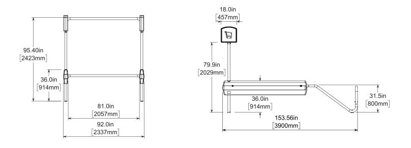
CartMagnet With Barriers CM-3B-COLOR Material: Galvanized Steel, High Density Polyethylene Cart Capacity: 30–36
